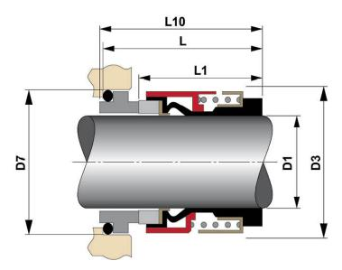
Mechanical seal "DYNAMICA" model DS-BH12/16 is widely used for GRUNDFOS-PUMP.
