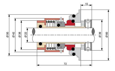
Mechanical seal "DYNAMICA" model DS-CRH22 is widely used for GRUNDFOS-PUMP. Balanced, cartridge O-ring seal unit with rigid torque transmission system. This seal type is assembled in a cartridge unit which makes replacement safe and easy. The balancing makes this O-ring seal type suitable for high-pressure applications.
