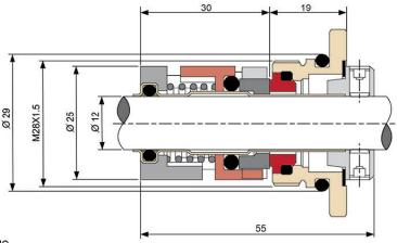
Mechanical seal "DYNAMICA" model DS-CRH12/16 is widely used for GRUNDFOS-PUMP. Balanced, cartridge O-ring seal unit with rigid torque transmission system. This seal type is assembled in a cartridge unit which makes replacement safe and easy. The balancing makes this O-ring seal type suitable for high-pressure applications.
